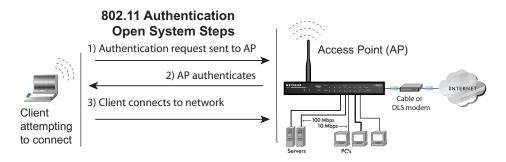
Figure 4-3: 802.11 open system authentication
